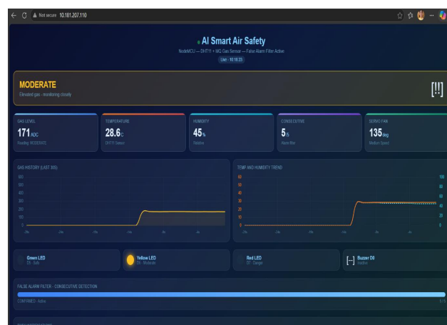
Fig. 6. Web dashboard displaying elevated gas readings under Moderate/Danger condition.
