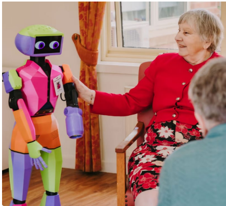
Fig. 1 Abi assistive robot for elderly care developed by Andromeda Robotics.
