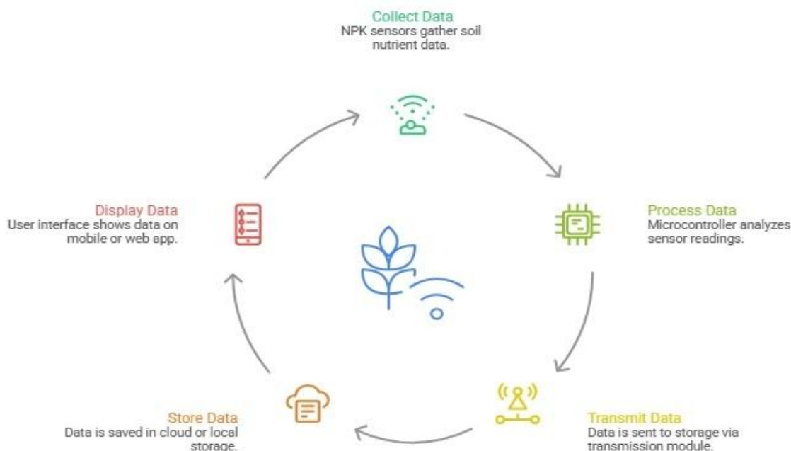
Fig.1 Real time NPK sensor monitoring cycle.
