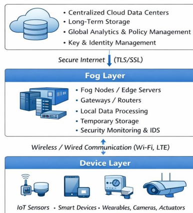
Figure 1. Fog Computing Architecture
