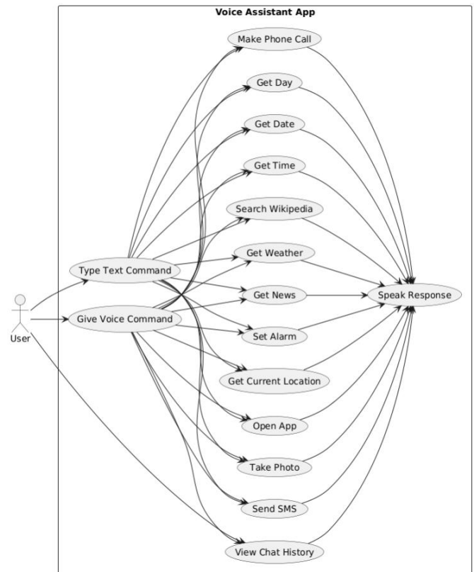
Fig 3: Use case diagram for Android Voice Assistant
